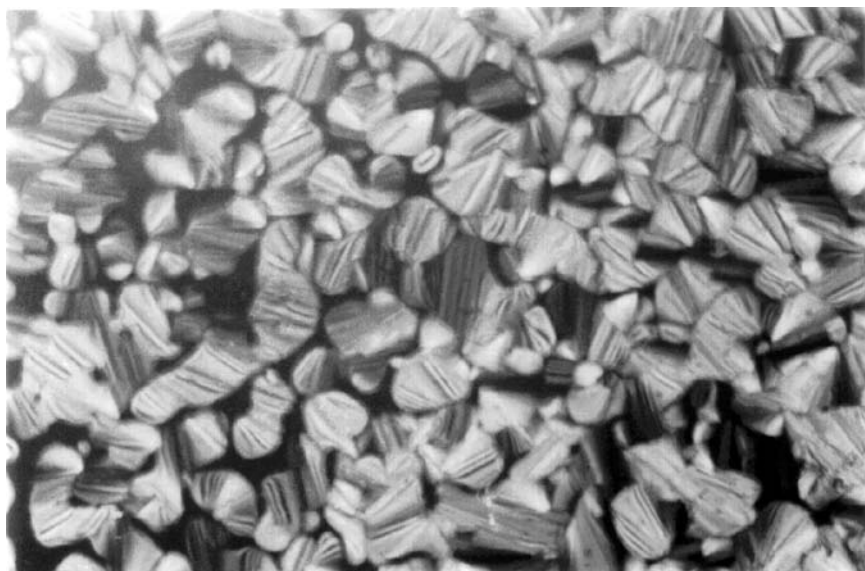
FIGURE 3 Photomicrograph of the texture of a binary 1:1 mixture of compound 5 and TNF obtained on cooling from the isotropic liquid at 200°C (crossed polarizers magnification \times 200 ). The texture resembles well the usual texture of columnar phase.
